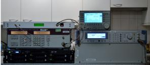
Figure 2: Backend (top left) with receivers, RAID server and Rubidium clock
