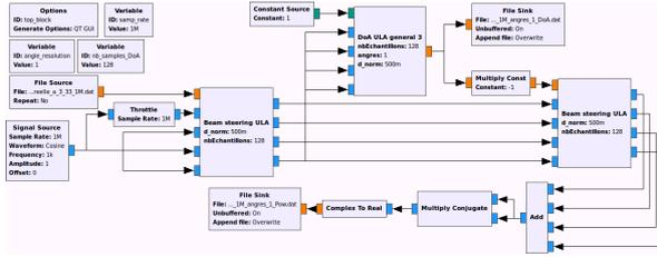
Figure 2: GNU Radio Companion flowgraph to simulate tracking of a fired projectile.
